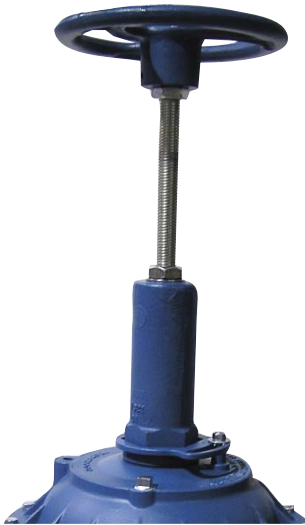
HWC Handwheel Closing Device This accessory will limit the opening of the valve and can be closed manually with the handwheel. Available with fail open and double-acting actuators, #25 and larger.
